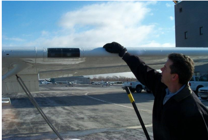
Figure III-6-1. Post application inspection can be critical for revealing any frozen contamination (Image reproduced by kind permission of the National Aeronautics and Space Administration (NASA).)
