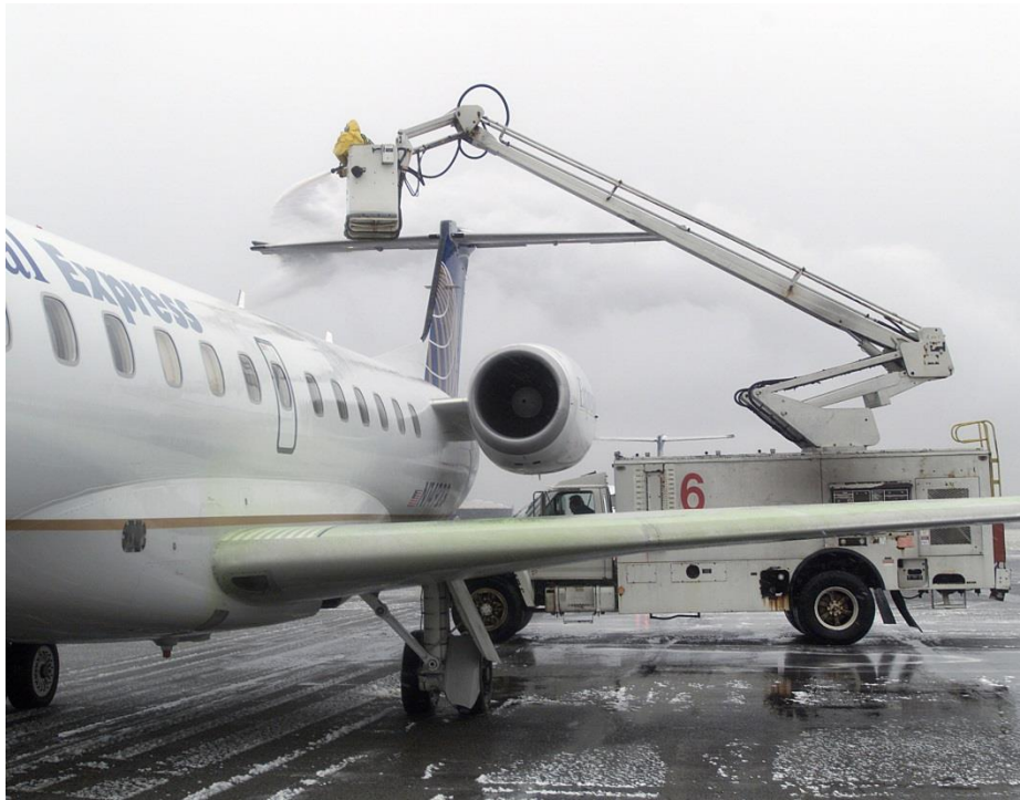
Figure III-10-1. Typical de-icing/anti-icing ground equipment (Image reproduced by kind permission of the National Aeronautics and Space Administration (NASA).)
